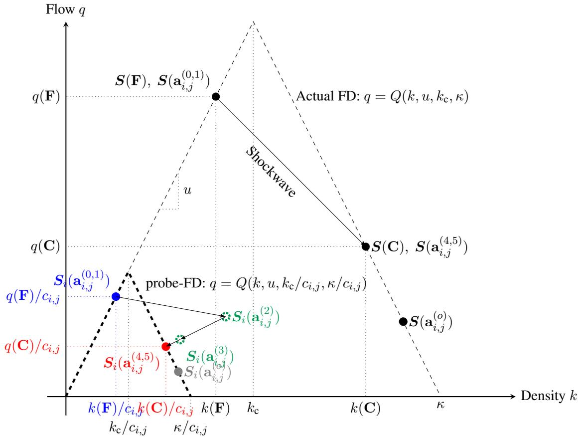
Figure 2: Traffic states transition on flow–density plane
